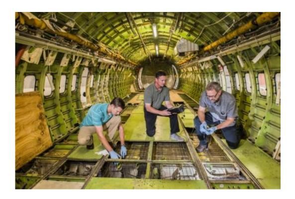
Sandia National Laboratories senior scientist Dennis Roach, center, works inside the cabin of a B737 test bed, installing and acquiring data from Structural Health Monitoring sensors with Sandia mechanical engineers Stephen Neidigk and Tom Rice. Credit: Randy Montoya
