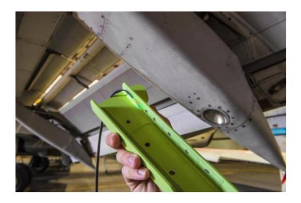
The Structural Health Monitoring sensors are custom built to fit an aircraft's parts. They can be mounted in hard-to-reach areas of an aircraft so that mechanics can plug in to acquire data without the time, cost and risk of removing parts from the aircraft. Credit: Randy Montoya
