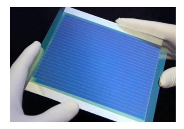
Imec's novel fullerene-free OPV cell concept was used to process an OPV module (156cm2) with a conversion efficiency of 5.3 percent.
