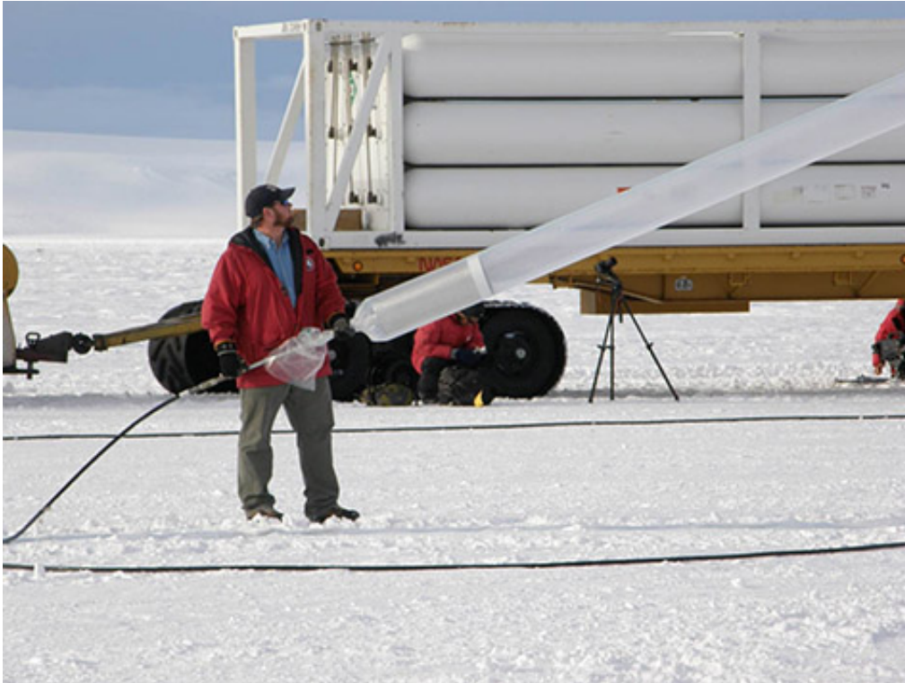
Closeup of a helium-carrying Kelly truck and a fill tube. Credit: NASA
