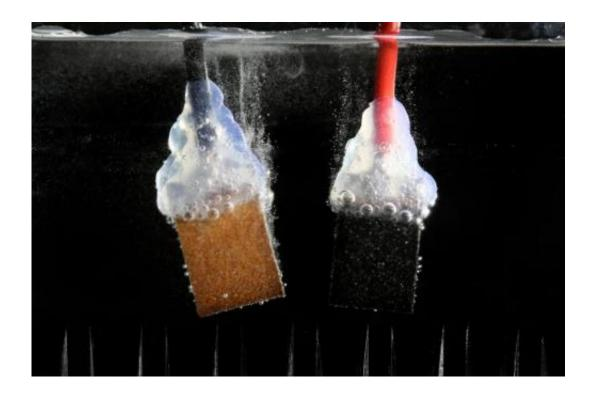
When an electrical current is provided, water splits into oxygen and hydrogen. Credit: EPFL / LPI / Alain Herzog
