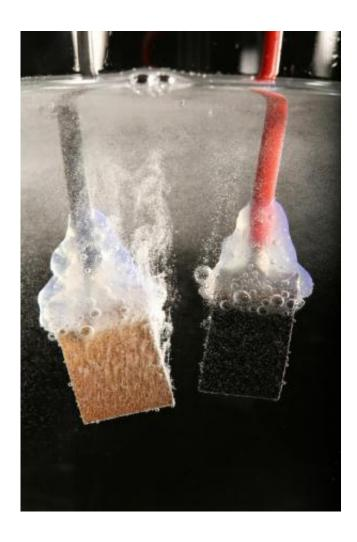
When an electrical current is applied, water splits into hydrogen and oxygen.
