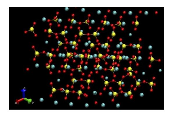
The generic molecular structure of cement consists of silicon (yellow) calcium (blue) and oxygen (red) atoms, with the addition of water molecules (not shown). A team of scientists including Rouzbeh Shahsavari of Rice University has created computational models to help concrete manufactures fine-tune mixes for specific applications Credit: Shahsavari Lab/Rice University
