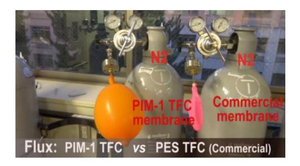
PIM-1 is a highly permeable membrane compared with commercially available ones. The orange balloon on the left illustrates this point as a higher volume of nitrogen gas is able to pass through PIM-1 into the balloon compared with the membrane on the right, connected to the pink balloon. Credit: Kyoto University
