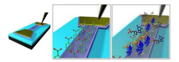
An illustration of an epitaxial graphene channel biosensor for detection of targeted 8-hydroxydeoxyguanosine (8-OHdG) biomarker. (A) Schematic of MLEG device (B) Thin film of covalently attached nitro phenyl (PhNO2) groups on the MLEG channel. (C) Attachment of the 'bioreceptor' antibody anti-8-OHdG to the amine terminated MLEG channel and subsequent detection of 8-OHdG. Credit: *2D Materials*
