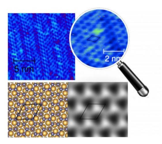
This is a 16.2 nm × 16.2 nm STM image of the modulated honeycomb  $\sqrt{7}\times\sqrt{7}$  superstructure. Atomic structures (side and top views) and simulated STM images of three different models of germanene on the  $\sqrt{7}\times\sqrt{7}$  Au(111) surface. Credit: *New Journal of Physics*
