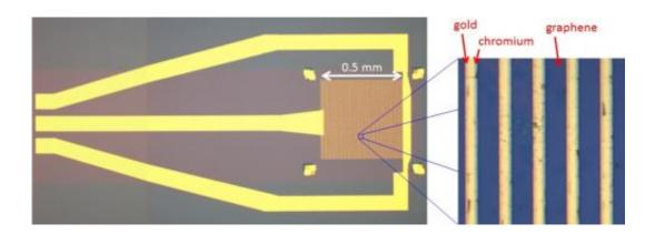
A graphene photothermoelectric detector. The active area of the device is a 0.5 mm by 0.5 mm square which consists of strips of graphene contacted by partially overlapping gold and chromium electrodes. Credit: Michael Fuhrer, Author provided
