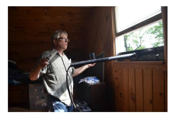
Lamont geochemist James Ross assembles an air sampler in an upstairs window of Beck's house. It will take background readings for a couple of weeks, before drilling starts.
