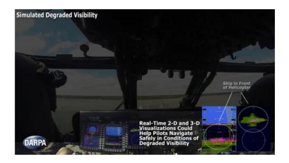
DARPA's Multifunction RF (MFRF) program seeks to enhance the survivability and combat effectiveness of helicopters facing degraded visibility. The program aims to develop multifunction sensor technology that would enable sensor packages small, light and efficient enough for installation on existing and future helicopter designs.
