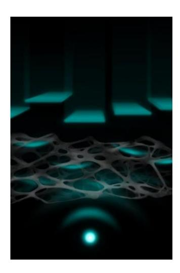
An artist's rendering of a shaped femtosecond pulse wavefront focusing through a scattering tissue. By pre-shaping the wave going into a complex scattering medium, it is possible to bring it to a sharp focus, enabling microscopy and other applications. Credit: Meital Covo
