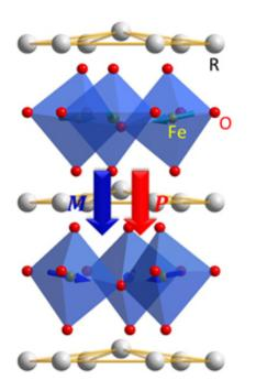
A schematic illustration of the crystal structure of h-RFeO3. The arrows on the Fe sites indicate the atomic magnetic moments. The coexisting spontaneous electric polarization (P) and magnetic polarization (M) are both along the same crystal direction. Credit: World Scientific Publishing
