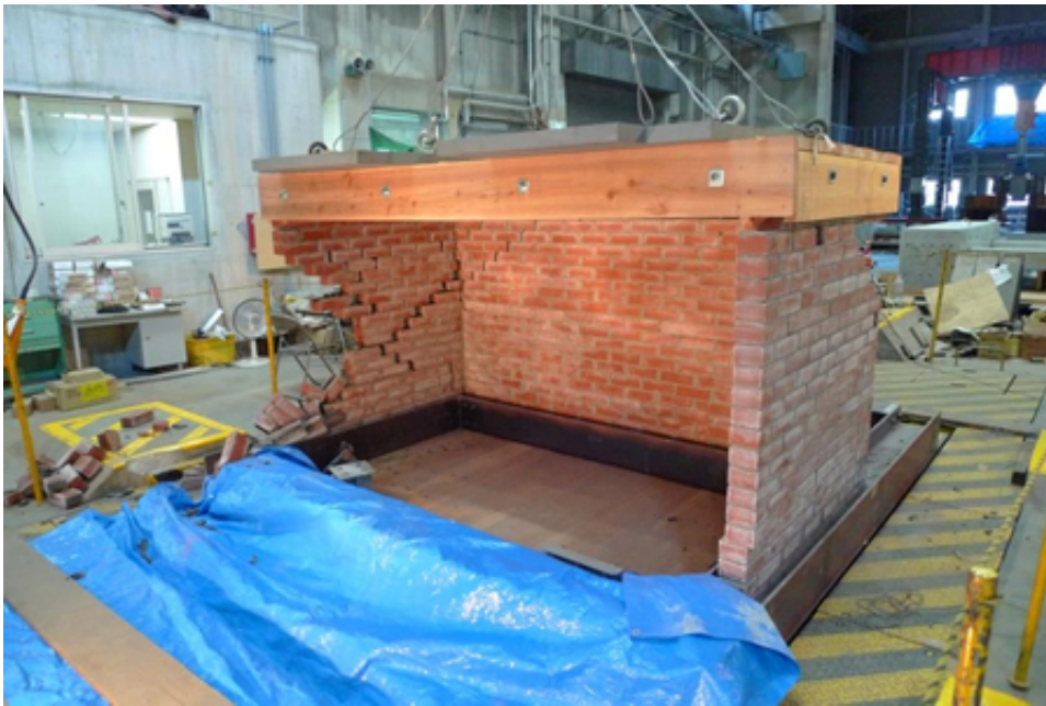
Fig.1: Collapse of the masonry wall specimen with a wooden slab.
