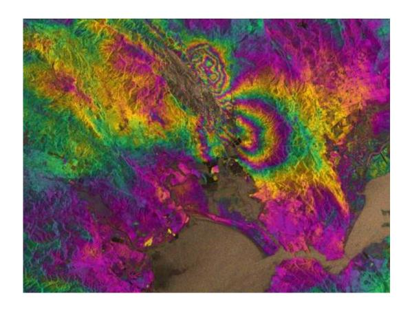
Interferogram of the Califorinia's Napa region created using two Sentinel-1A images. The two round shapes around Napa valley, which are visible in the central part of the image show how the ground moved during an earthquake on August 24, 2014. Credit: Copernicus data (2014)/ESA/PPO.labs/Norut/COMET-SEOM Insarap study
