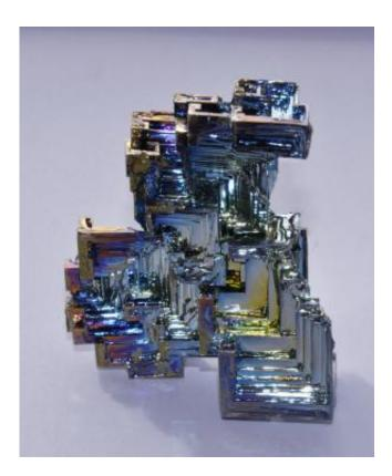
Semi-metallic bismuth crystal, used in thermoelectric compounds and special bearing alloys. Credit: ESA
