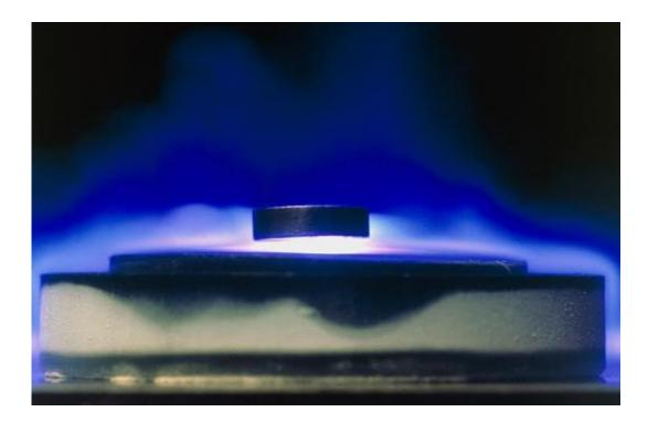
Magnetic levitation of a high-temperature 'cuprate' superconductor, caused by the Meissner effect, which causes the magnetic flux to be expelled from a superconductor. Credit: Birmingham University
