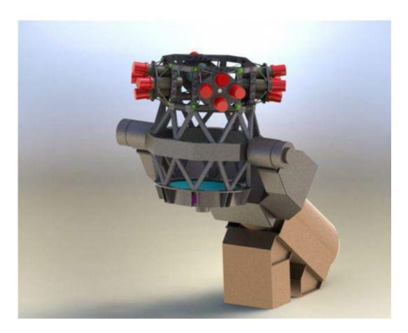
A new, European telescope nicknamed 'fly-eye' splits the image into 16 smaller subimages to expand the field of view, similar to the technique exploited by a fly's compound eye. Such fly-eyed survey telescopes provide a very large field of view: 6.7° x 6.7° or about 45 square degrees. 6.7° is about 13 times the diameter of the Moon as seen from the Earth (roughly 0.5 degrees). Credit: ESA/Compagnia Generale dello Spazio CGS
