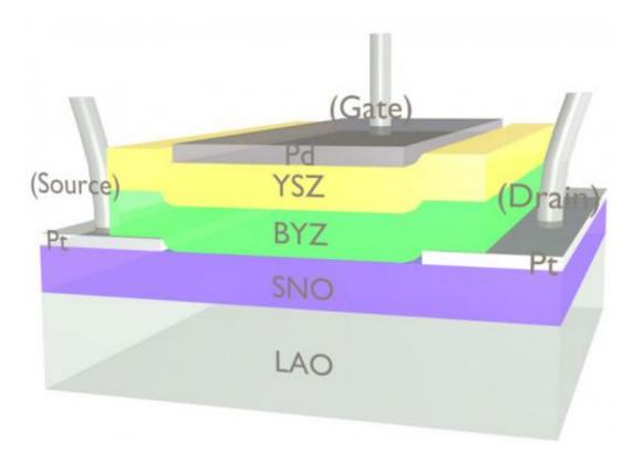
'This is a new type of correlated transistor where the transistor action is gated by an ionic field,' says principal investigator Shriram Ramanathan. Credit: Jian Shi.
