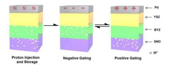
During fabrication, the annealing process injects hydrogen ions into thin films of samarium nickelate (SNO) and yttrium-doped barium zirconate (BYZ). During operation, an electric field moves the charges from one layer to the other, and the influx or loss of electrons modulates the band gap in the SNO, resulting in a very dramatic change in conductivity. Credit: Jian Shi.
