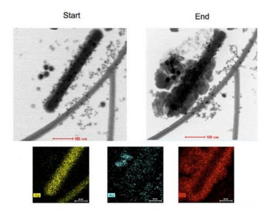
Techniques at Argonne's Electron Microscopy Center helped scientists get a complete picture of this chemical reaction. Over the course of the reaction, the nanorod on the top left is slowly covered with a growth of copper deposits from the solution. Maps showed the locations of the elements in the reaction: Ag, or yellow, representing silver; blue representing gold, Au; and Cu, copper, shown in red. Credit: Nestor Zaluzec / Argonne National Laboratory Electron Microscopy Center.
