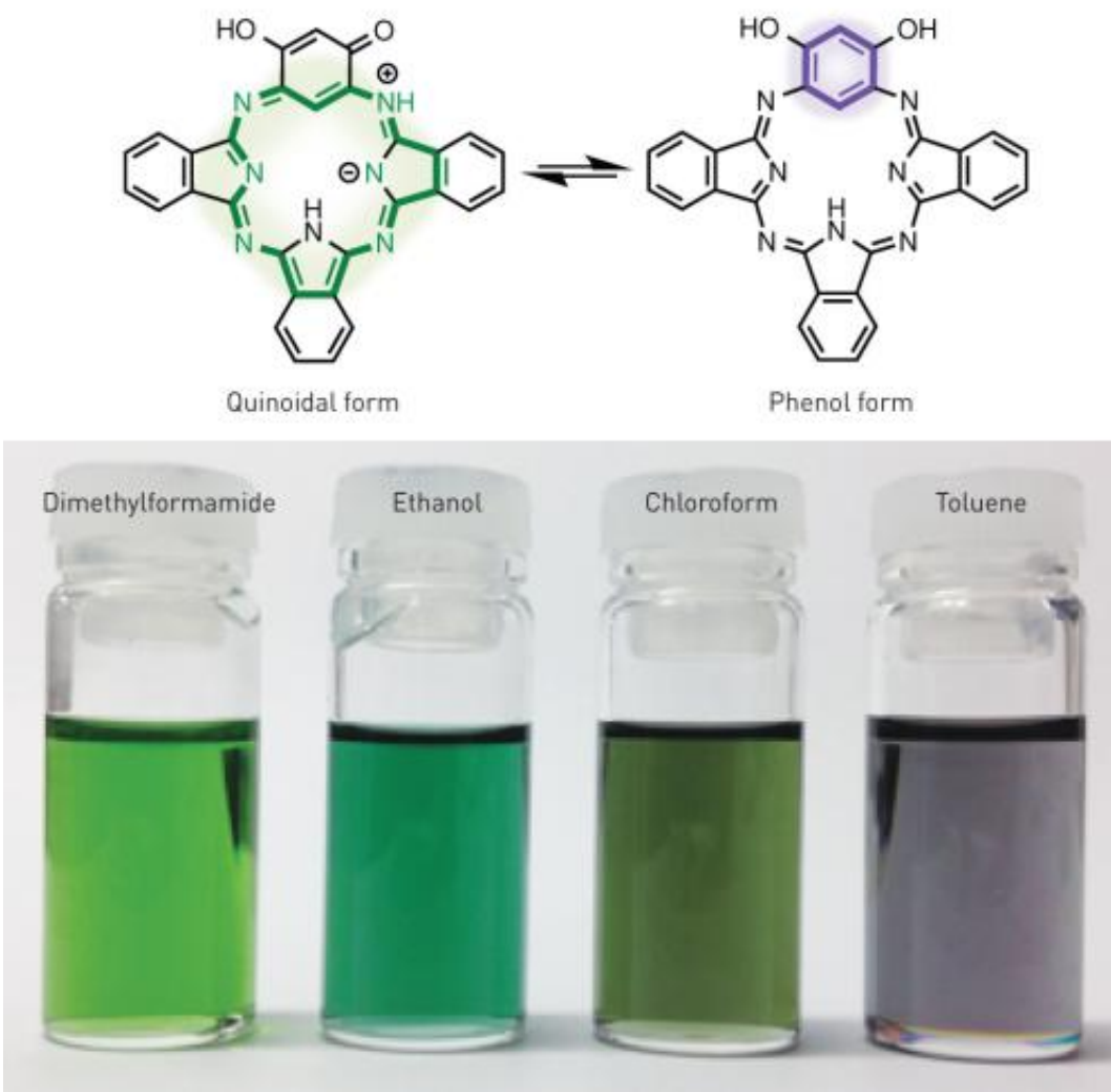
Figure 1: Different solvents can cause benzophthalocyanine to shift between its strongly aromatic quinoidal form and its weakly aromatic phenol form, which changes the color of the solution. Credit: Atsuya Muranaka, RIKEN Center for Sustainable Resource Science
