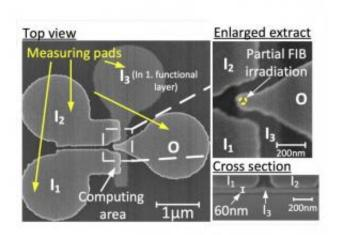
This image shows scanning electron micrographs of a 3-D majority logic gate showing the scale of the computing area ,with dimensions less than 200 nanometers, and, in cross-section, the lower position of the third input magnet. Credit: I. Eichwald/TUM
