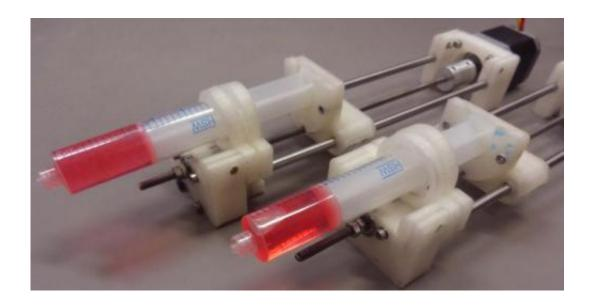
Researchers can now save thousands of dollars and slash the time it takes to complete experiments by printing parts for their own custom-designed syringe pumps. Members of Joshua Pearce's lab made this web-enabled double syringe pump for less than \$160. Credit: Emily Hunt
