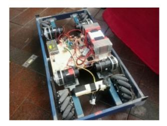
Under the couch's standard wood frame is a custom steel chassis fitted with four independently controlled mecanum wheels.
