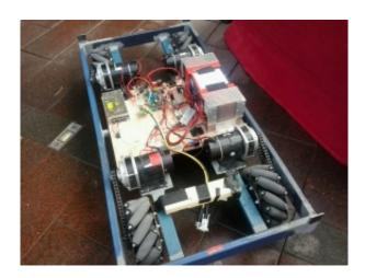
Under the couch's standard wood frame is a custom steel chassis fitted with four independently controlled mecanum wheels.
