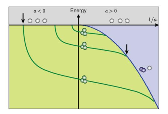
A graph of Efimov triplet states as a function of the scattering length, a, and the binding energy. Outside the green area the three cesium atoms exist singly or as a pair plus a lone atom. Credit: Image courtesy of the University of Innsbruck
