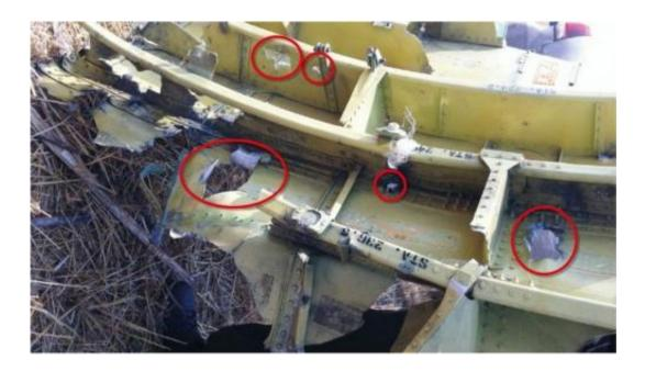
Part of the inside cockpit roof showing penetration by objects from outside. Credit: DCA/Dutch Safety Board
