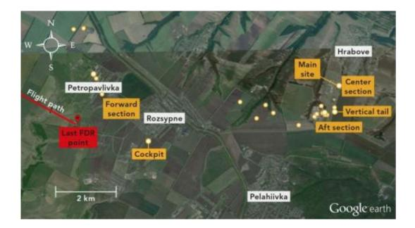
The last location of the aircraft in flight taken from the flight data recorder (FDR). Wreckage distribution is grouped per section of the aircraft. Credit: Dutch Safety Board
