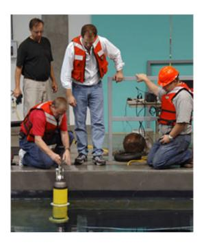
(from left to right) Ken Johnson, Dana Swift, Luke Coletti, and Hans Jannasch test a profiling float similar to the floats that will be used for SOCCOM in MBARI's test tank. Credit: MBARI.
