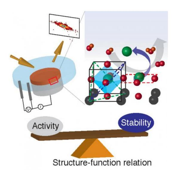
Left: Schematic of in situ x-ray studies conducted at the APS for oxygen evolution reaction. A cylindrical sample, SrRuO3 (red) on Nb:SrTiO3 (gray) is exposed to a thin electrolyte layer (blue, 0.1 M KOH). Right: The model system [SrRuO3 (001)-red, (110)-blue, and (111)-green dashed line] produces oxygen
