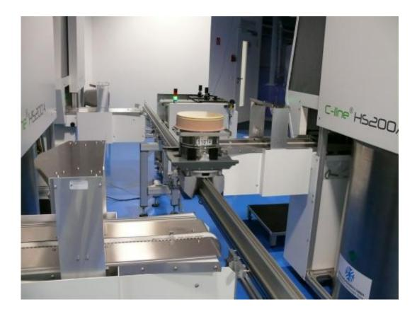
The biobank comprises three cryotanks, equipped with cooled protective hoods, and a transfer station from which the sample containers are transported via a rail system. There is enough space for approximately 60,000 samples. Credit: Fraunhofer IBMT
