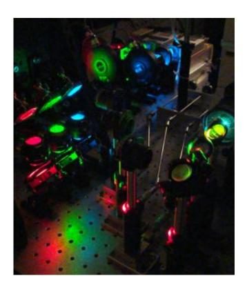
This is atotal internal reflection fluorescence (TIRF) microscope used in Charles Asbury's lab at the University of Washington, where his team studies the molecular machinery of chromosome separation during reproductive cell division. Credit: Charles Asbury
