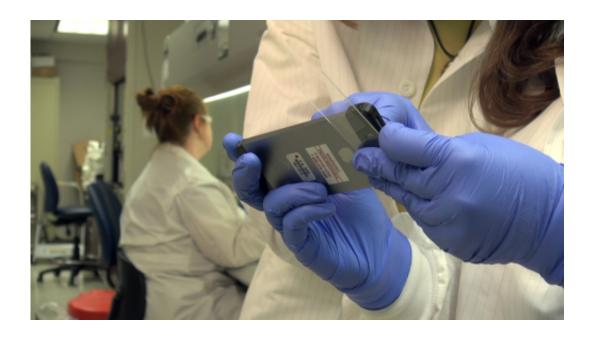
Researchers look at simulated anthrax spores through a 1000x microscope created on a 3D printer that attaches to a cell phone.
