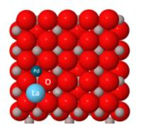
Space filling model for the La and Pd on the g-alumina (100) surface. Atoms are: oxygen/red, aluminum/gray, palladium/dark blue, and lanthanum/light blue. The La atoms sit in the four fold hollows on the alumina surface and help to trap the Pd atoms nearby.
