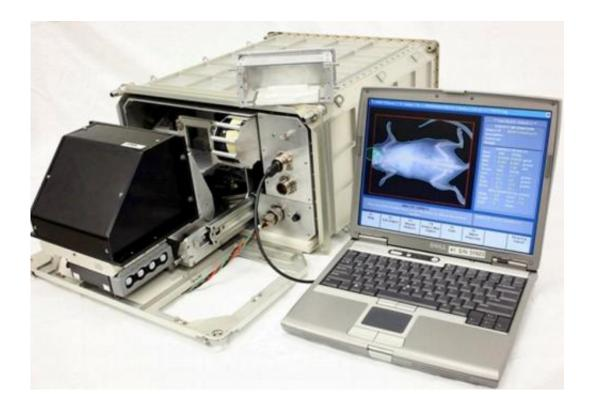
The Bone Densitometer developed by Techshot, Inc. will enable X-ray testing for research studies aboard the International Space Station. Credit: CASIS
