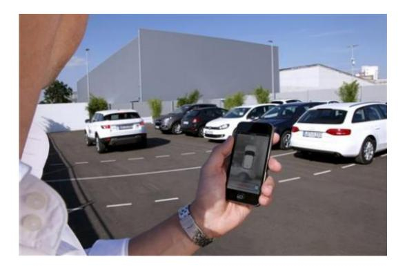
In this undated photo supplied by Valeo, a person activates a self-parking vehicle via a smartphone application. Technology being honed by the French auto parts maker uses a dozen ultrasonic sound-wave sensors, 360-degree cameras and a laser scanner to allow a vehicle to safely park within a few centimeters of other vehicles. (AP Photo/Valeo)
