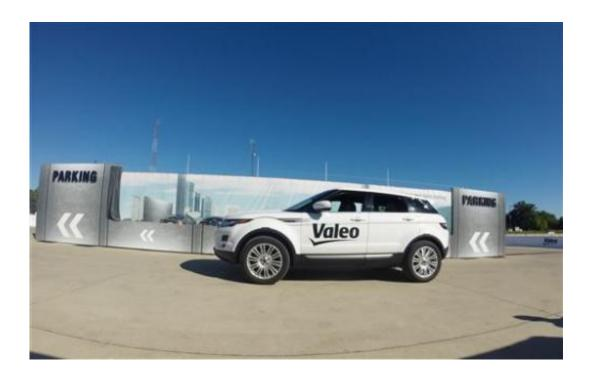
A Range Rover drives by itself toward a parking spot during a demonstration by Valeo on Sept. 8, 2014, in Detroit. Technology being honed by the French auto parts maker uses a dozen ultrasonic sound-wave sensors, 360-degree cameras and a laser scanner to allow a vehicle to safely park within a few centimeters of other vehicles. (AP Photo/Mike Householder)
