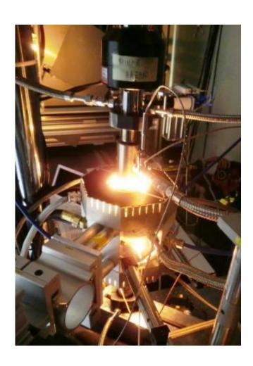
A mechanical stress testing setup with a custom-built compact furnace and cooling system that mimic extreme operating conditions on turbine engines at the Advanced Photon Source at Argonne National Laboratory. Credit: DLR
