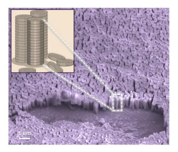
Vertical nanopillars are ideal geometries for getting around the challenges of producing polymer architecture to boost power-conversion efficiency of light to electricity to power electronic devices. Credit: UMass AMherst
