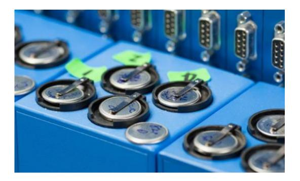
An apparatus used to charge lithium ion coin cell batteries at various rates with different levels of current at the Stanford Institute for Materials Science and Engineering. The results indicate that the benefits of slow draining and charging may have been overestimated. Credit: SLAC National Accelerator Laboratory
