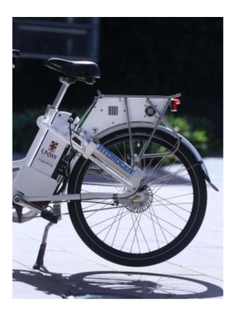
Close-up of the hydrogen canister and fuel cell.
