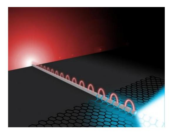
Far-field photons excite silver nanowire plasmons. The wire plasmons propagate to the wire's distal end where they efficiently interact with the two-dimensional material semiconductor molybdenum disulfide (MoS2). The plasmons are absorbed in the MoS2 creating excitons that subsequently decay converting back into propagating photons. Credit: Michael Osadciw, Creative Services, University of Rochester
