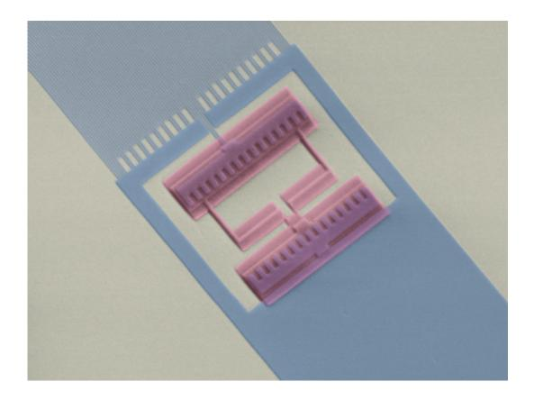
Microscope image: This is a zoom-in of the artificial atom, with its integrated Superconducting Quantum Interference Device (SQUID) in violet. The SQUID gives the atom its quantum properties, and the fingers sticking up to the left provide the coupling to sound waves. Credit: Martin Gustafsson and Maria Ekström
