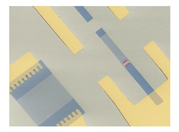
Microscope image: The artificial atom, in grey-blue to the upper right, can emit and absorb sound that moves across the surface of a microchip. The grey-blue structure to the lower left is the combined loudspeaker/microphone used to communicate acoustically with the atom. Credit: Martin Gustafsson and Maria Ekström
