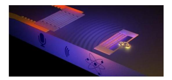
On the right, an artificial atom generates sound waves consisting of ripples on the surface of a solid. The sound, known as a surface acoustic wave (SAW) is picked up on the left by a "microphone" composed of interlaced metal fingers. According to theory, the sound consists of a stream of quantum particles, the weakest whisper physically possible. The illustration is not to scale. Credit: Philip Krantz, Krantz NanoArt
