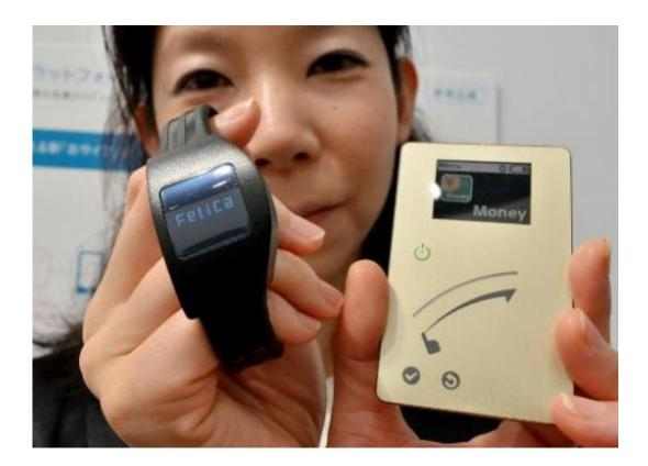
Sony's prototype model of a smart card with a NFC chip (R) which has a LCD display enabling users to check the account balance, electronic coupon and other electronic information and a wrist watch shaped device, seen in Tokyo, on July 17, 2014
