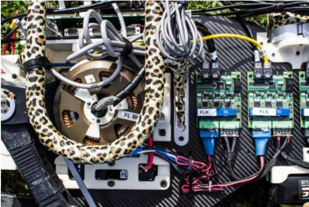
The custom, high-torque-density motors and amplifier. Credit: Jose-Luis Olivares/MIT
