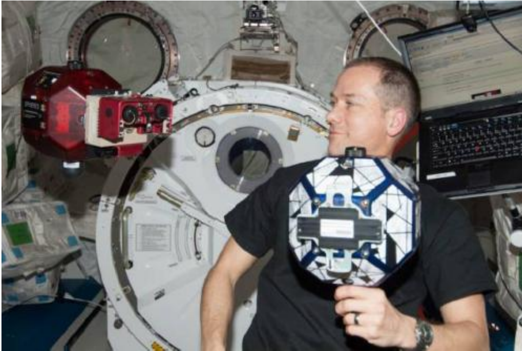
SPHERES satellites with Goggles onboard ISS. Credit: MIT Space Systems Laboratory and the researchers
