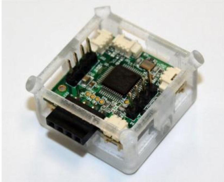
The D-Board, the general sensor/processor platform developed for the prototype system.
