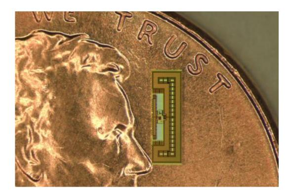
The tiny radio-on-a-chip gathers all the power it needs from the same electromagnetic waves that carry signals to its receiving antenna.
