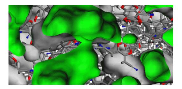
Polymer molecular sieves with interconnected pores (in green) for rapid and selective transport of molecules. Credit: Qilei Song
