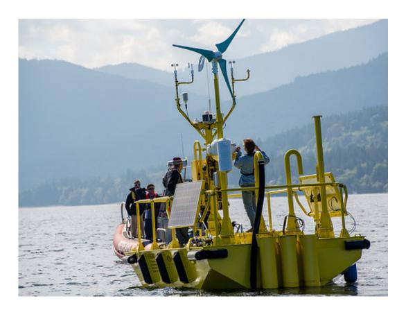
Research on the High Seas: Pacific Northwest National Laboratory staff conduct tests in Sequim Bay, Washington, while aboard one of two new research buoys being commissioned to more accurately predict offshore wind's power-producing potential.
