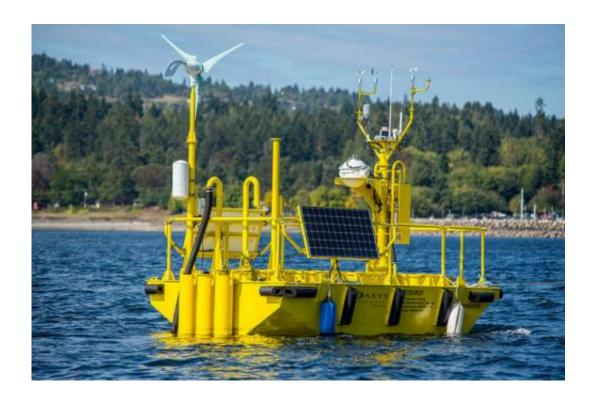
Blowin' in the Wind: Pacific Northwest National Laboratory is commissioning two of these large buoys, which are decked out with advanced scientific instruments to more accurately predict offshore wind's power-producing potential.
