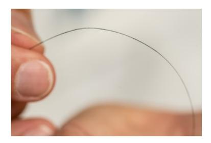
Fiber of pure carbon nanotubes has potential for use in small-scale electronics and large scale power applications. Credit: Jeff Fitlow
