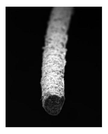
Carbon nanotubes extruded into a pure fiber are the product of an acid-free process invented at Rice University. Credit: Martí Group
