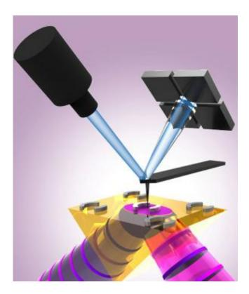
Schematic showing the photothermal induced resonance (PTIR) technique, which combines the lateral resolution of atomic force microscopy (AFM) with the chemical specificity of IR spectroscopy. A wavelength-tunable, pulsed IR laser (purple) illuminates a sample consisting of plasmonic gold resonators from the below. The resulting thermal expansion of the sample is detected locally by the AFM cantilever tip, which is monitored by reflecting a laser (blue) off the back of the cantilever.
