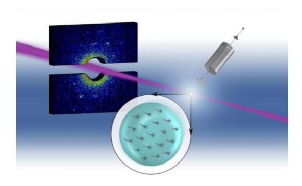
This is an illustration of analysis of superfluid helium nanodroplets. Droplets are emitted via a cooled nozzle (upper right) and probed with x-ray from the free-electron laser. The multicolored pattern (upper left) represents a diffraction pattern that reveals the shape of a droplet and the presence of quantum vortices such as those represented in the turquoise circle with swirls (bottom center). Credit: Felix P. Sturm and Daniel S. Slaughter, Berkeley Lab.
