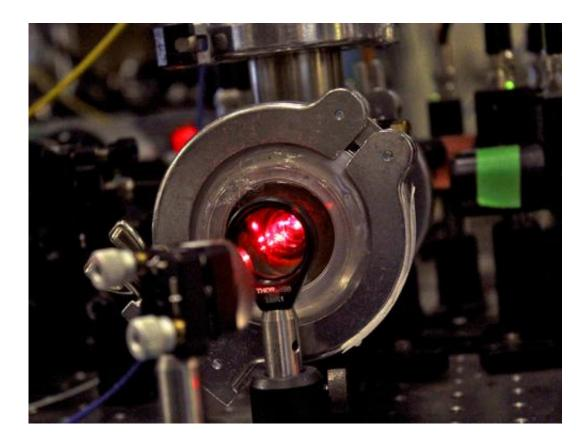
An optical cavity was used to control the wavelength of some of the lasers used for the magneto-optical trap. Credit: Michael Helfenbein
